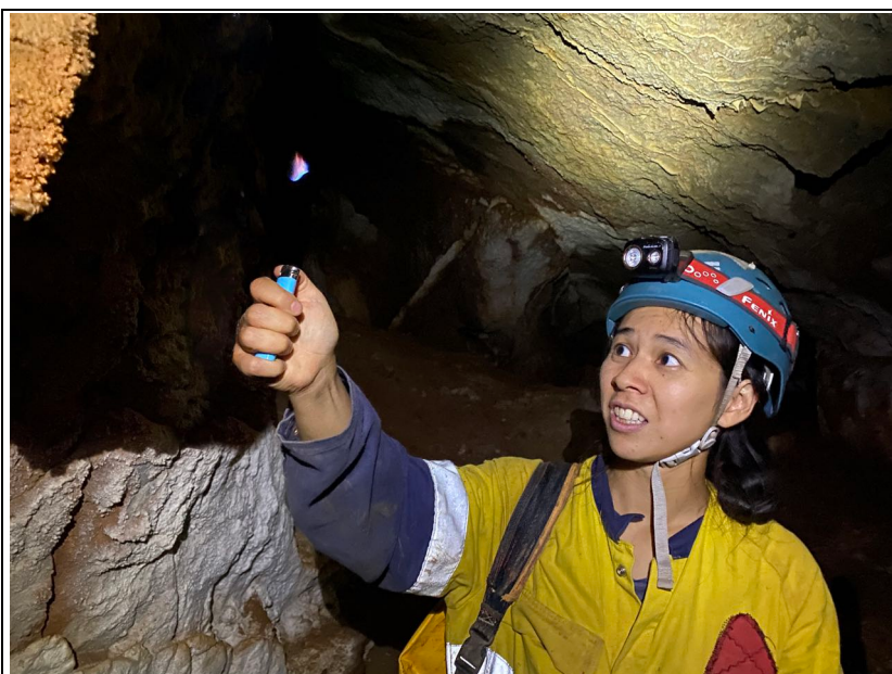
Fig 3. Cindy Li performing a party trick demonstrating the foul air interface in Moores Cave Timor. When the cigarette lighter flame is lit in good air the flame extends directly from the lighter jet. As the lit cigarette lighter is then lowered into a layer of foul air, the flame remains burning in air which can just support combustion. Keep lowering the cigarette lighter and the flame will extinguish.
