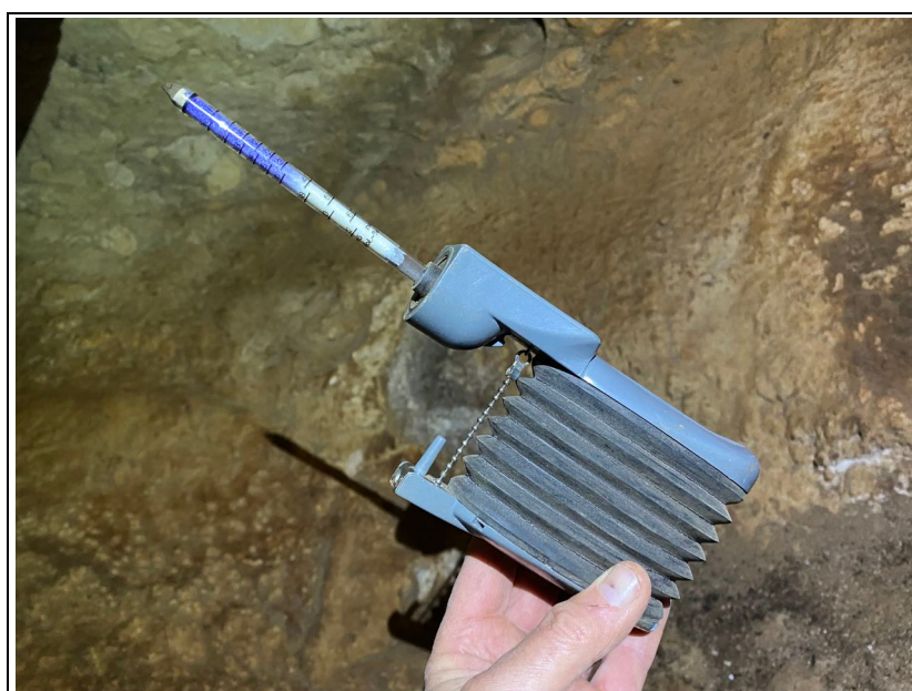
Fig 4. Dräger-Tube gas analyser is showing by the change in tube colour to purple, that there is a 4% CO 2 concentration in Moores Cave, Timor, NSW.
